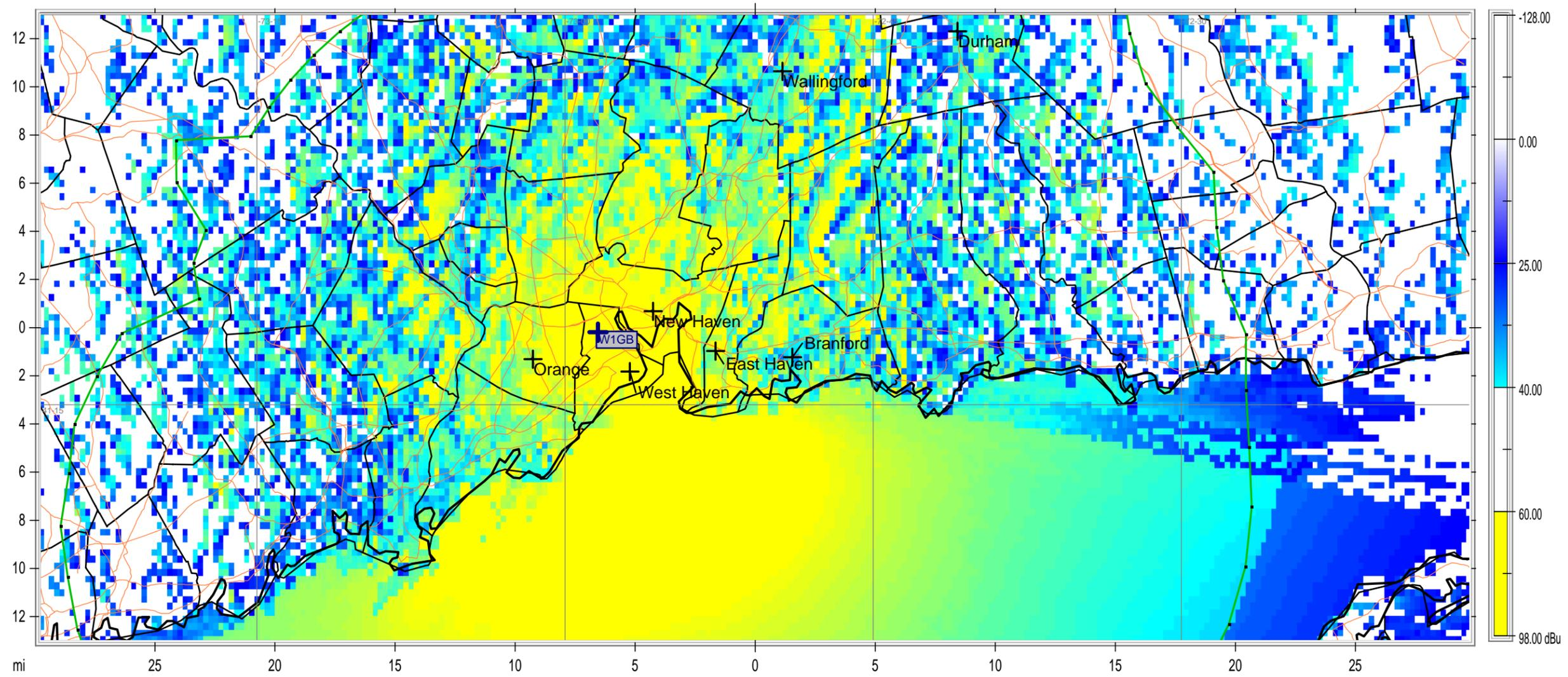
146.61 Repeater Talk-out @ 275 watts ERP 25 dBu Min FS
